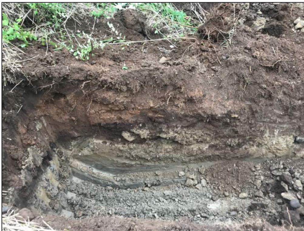
Image 5. Subsurface conditions in test pit TP-3 showing surficial brown fill with debris, dark brown relict topsoil, and tan, very stiff clay.
