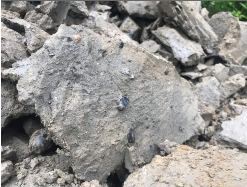
Image 6. Test pit TP-4 spoils from approximately 8 feet BGS. Note scattered gravel (dropstones) in clay matrix often indicative of glaciomarine drift soils.
